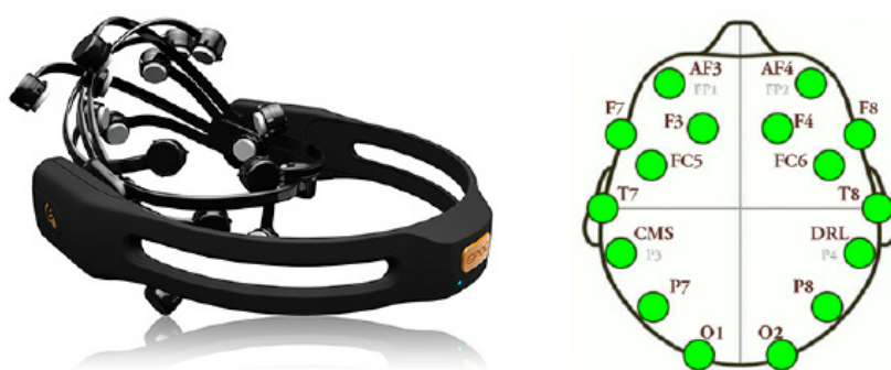
Figure 7. Emotiv Epoc+ headset and electrodes location (Emotiv, San Francisco, CA, USA).
